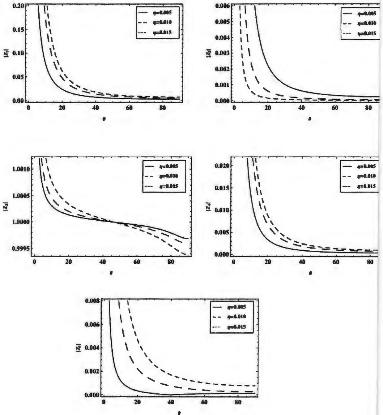
Fig. 3.4: Variation of amplitude with  $|Z_i|$  (1, 2, ..., 5) with the angle of incidence of SV-wave for variation of viscosity.
