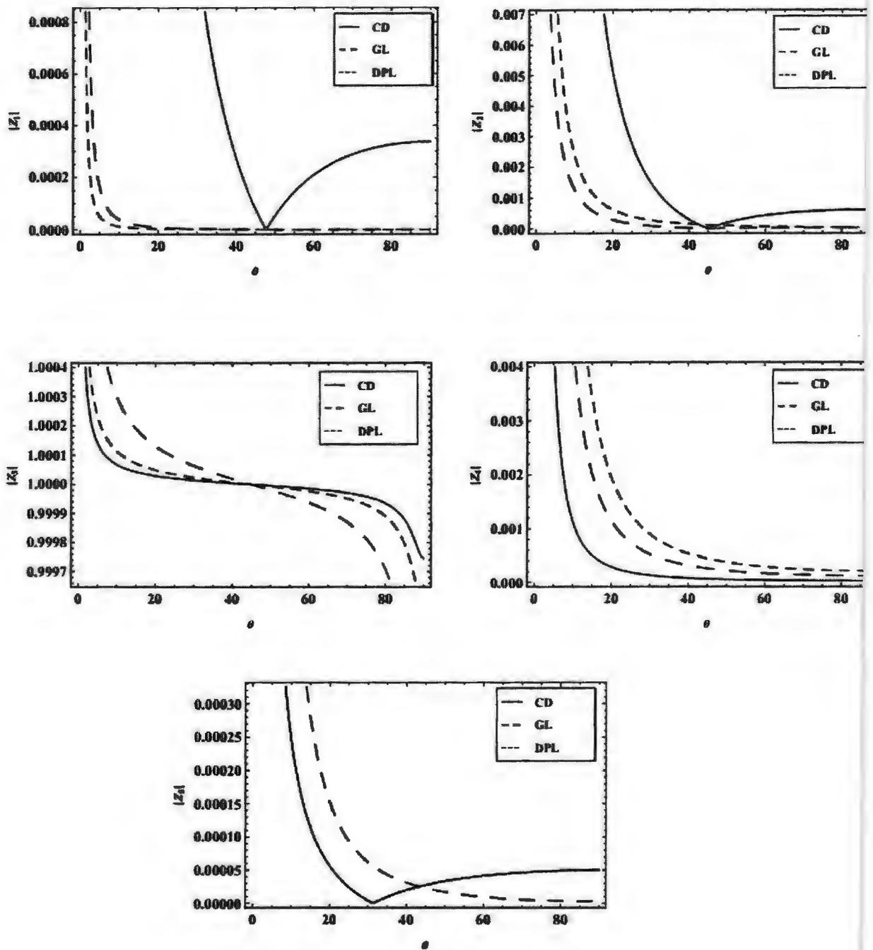
Fig. 3.3: Variation of amplitude with  $|Z_i|$  (1, ..., 5) with the angle of incidence of SV-wave in absence of gravity
