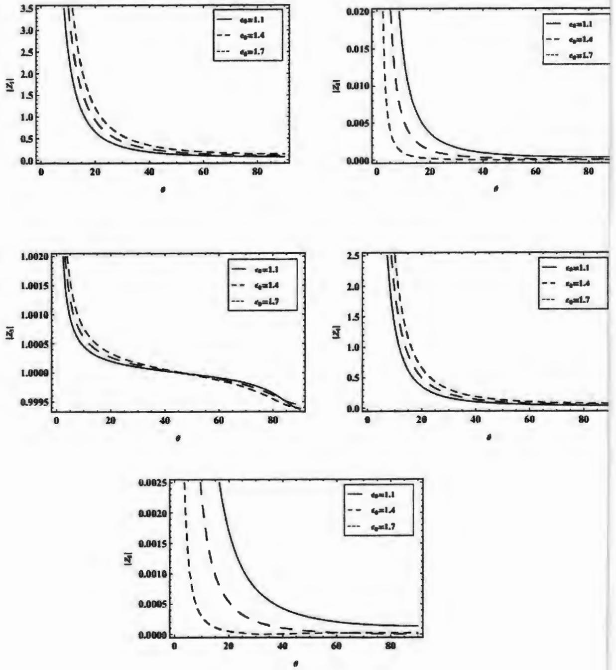
Fig. 3.7: Variation of amplitude with  $|Z_i|$  (1,.....5) with the angle of incidence of SV-wave for variation of magnetic field.
