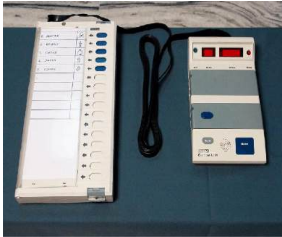
(This figure showing Control unit on the Right side and the Balloting unit on the Left side)
