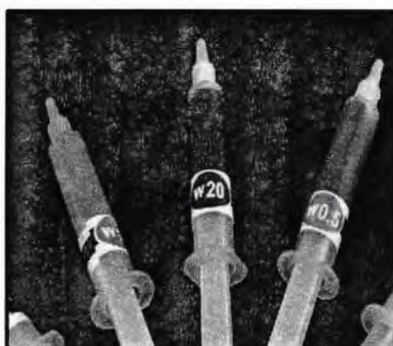
Fig. 3.6 Rough and fine diamond crystal paste
