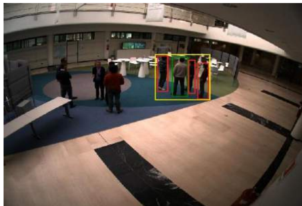
Figure 4.2: illustration of selection of interacting persons under d^{th} . Green rectangle is drawn around focal person. The threshold area around focal person is represented with yellow rectangle. The persons detected under d^{th} are marked with red rectangle.
