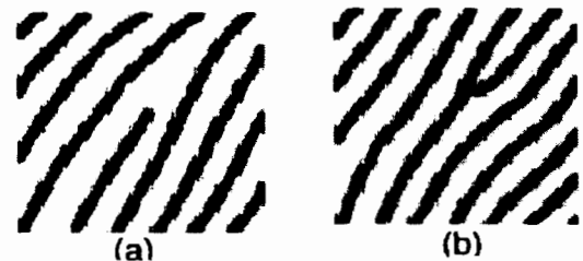
Fig. 1: Two most widely used minutia features a) Ridge Ending b) Ridge Bifurcation
