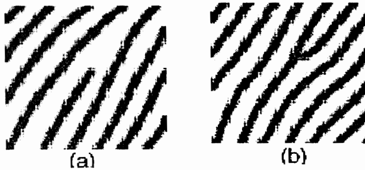
Figure 2.3 Two most widely used minutia features a) Ridge Ending b) Ridge Bifurcation
