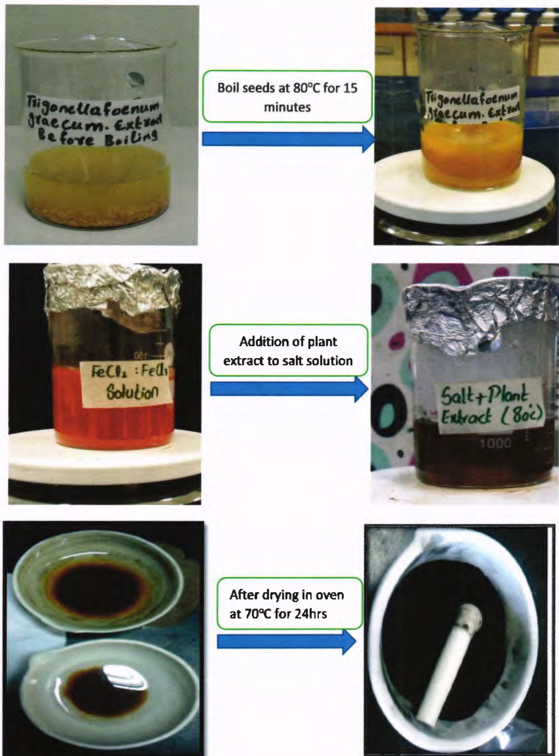
Fig.2.3 Plant mediated synthesis of Iron Oxide Nanoparticles
