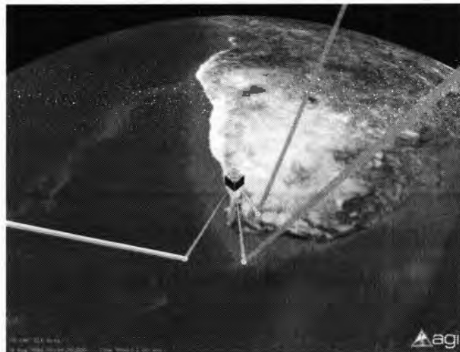
Figure 4-12: Bistatic reflection geometry for signals from three GNSS satellites received in LEO
