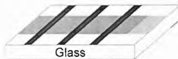
Figure 2.10: Deposition of Electrical contacts (Al)
