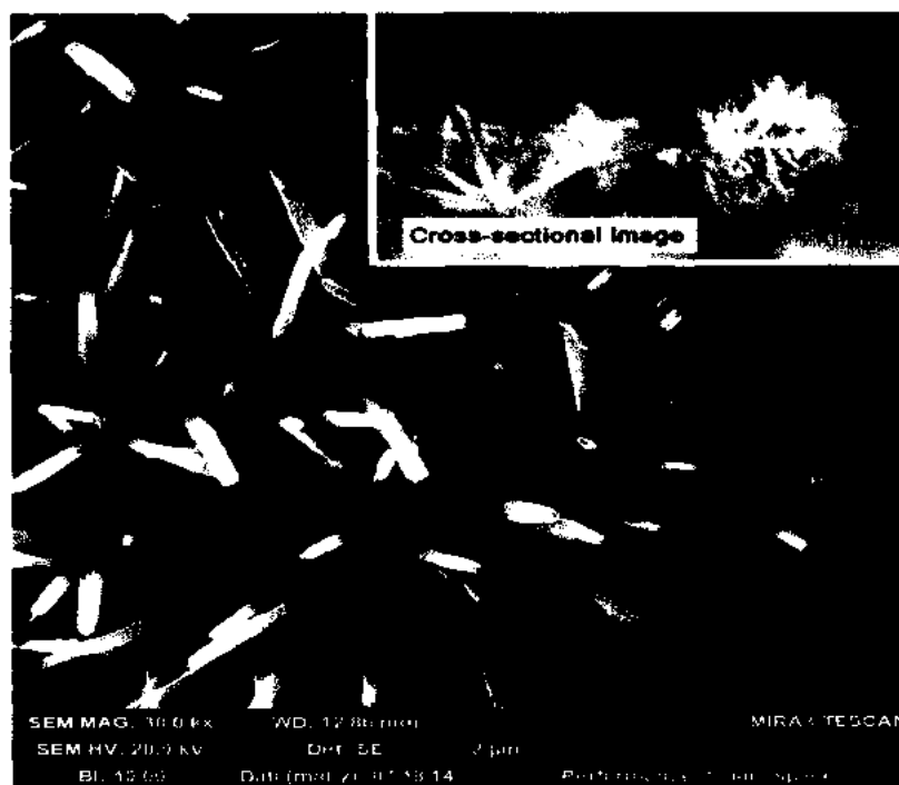
Figure 4.8: SEM image of Al-doped ZnO nanorods grown on uncoated glass substrate.
