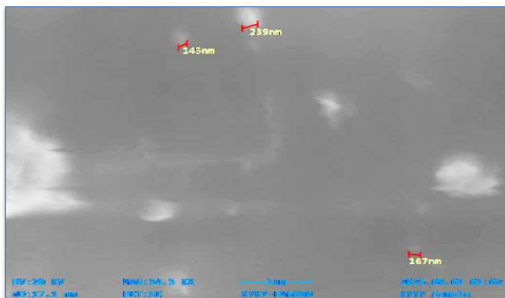
Figure 4.9 SEM analysis of Zn-Cobalt Oxide NPs at different magnification (30-1000X)
