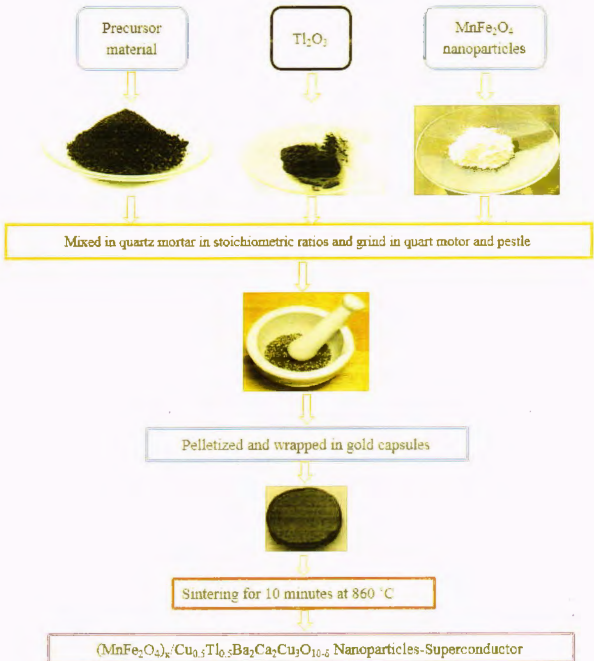
Fig. 3.4: complete flow diagram of preparation of (\text{MnFe}_2\text{O}_4)_x/\text{Cu}_{0.5}\text{Tl}_{0.5}\text{Ba}_2\text{Ca}_2\text{Cu}_3\text{O}_{10.5} Nano-Superconductor.
