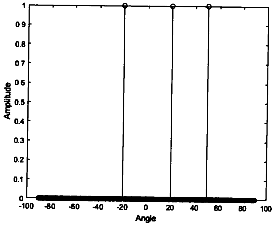
Fig 5.10: Detection of three sources with added noise of -40dB
