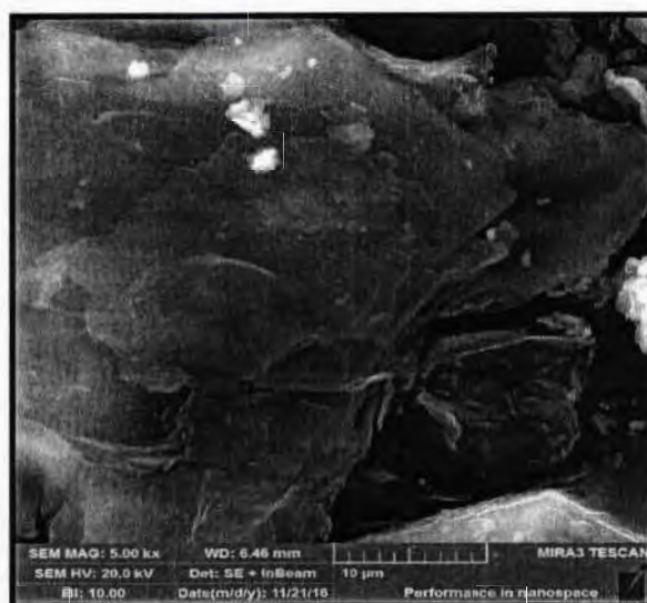
Figure 23: SEM image of MgO/GO nanocomposites with 10% dispersion
