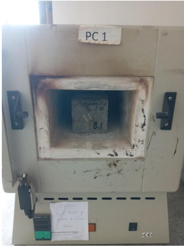
Figure 3-7: Heating of concrete specimen in the Muffle furnace
