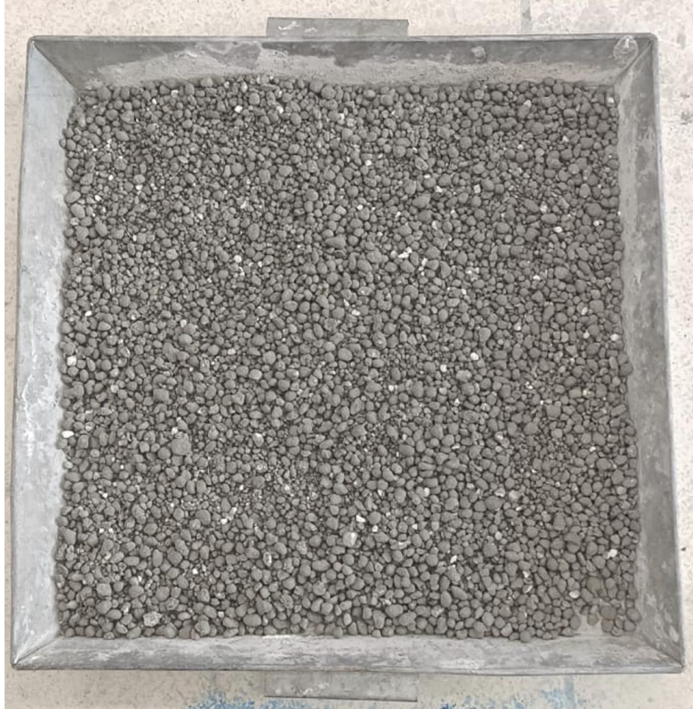
Figure 3-4: Preparation of Granules in a batch
