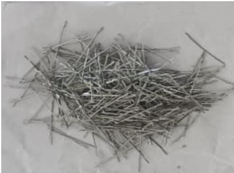
Figure 3-3: Steel Fibers as provided by the vendor
