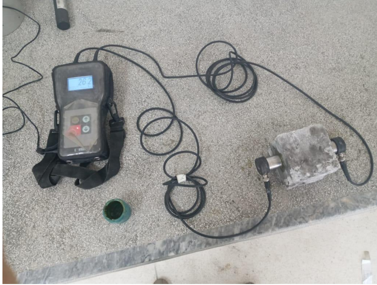
Figure 3-10: UPV testing of the specimens
