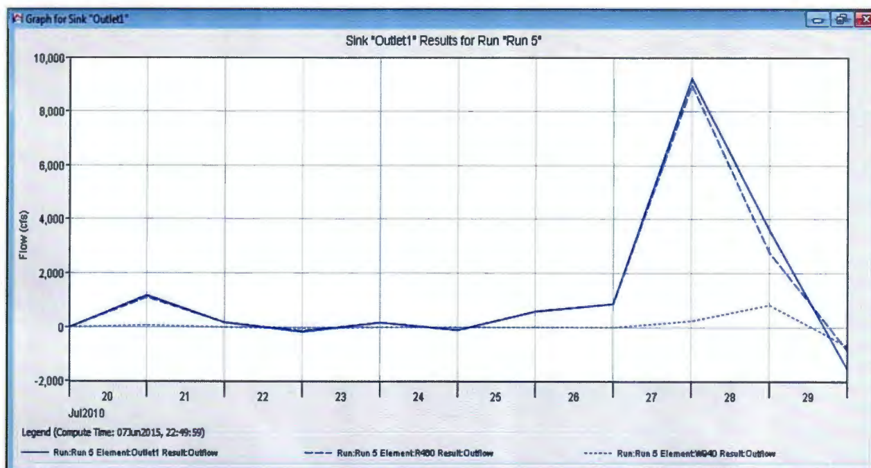
Fig 3.14: Graph for sink showing the difference between the outflow of hydrologic elements i.e. Outlet, Reach (R) and Subbasin (W).
