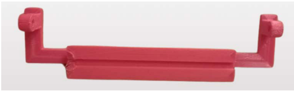
Figure 16 3D printed rotary heater frame fabricated via FDM using PLA.
