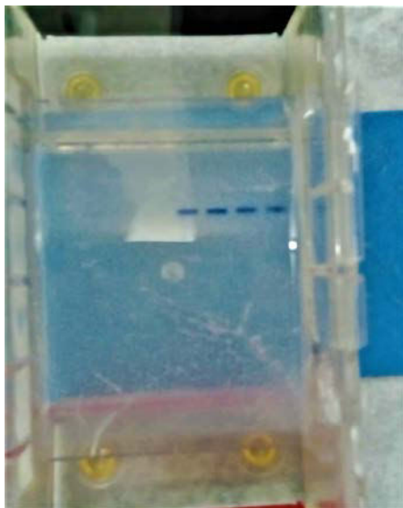
Figure 31 Agarose gel electrophoresis showing PCR amplification results of Plasmodium vivax DNA. Lane 1: Positive control amplified using commercial thermocycler; Lanes 2–4: DNA amplified using the developed thermal cycling device.
