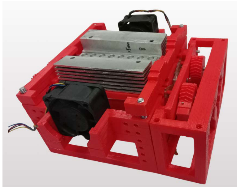
Figure 28 Assembly of key components on the PCR device base and CAN machined components and cooling fans mounted above.
