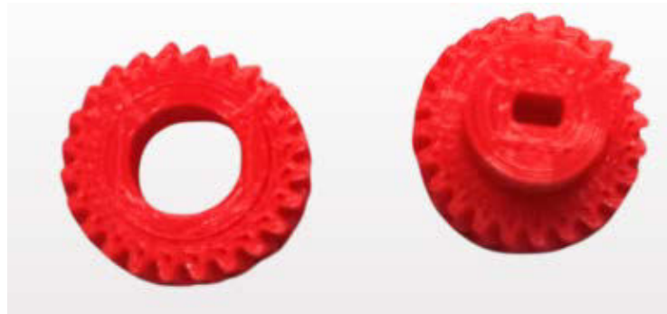
Figure 20 FDM-printed gear system optimized for torque and synchronization.
