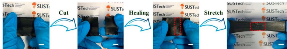
Fig 3.21: Strain sensor nano-composite shows healing and stretching property [144]
