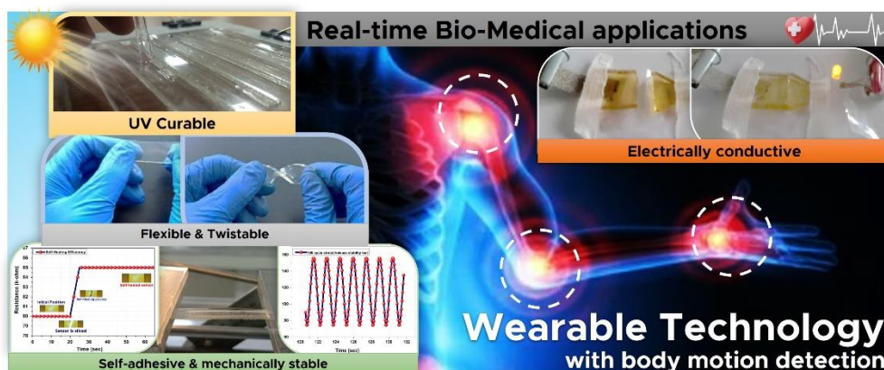
Fig 5.26: Proposed strain sensor represented real time graphical body motion detection
