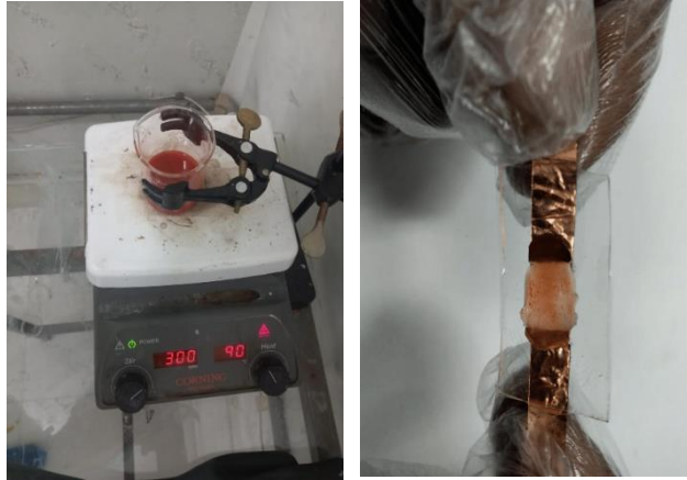
Fig 5.8: Physical fabrication of sensor: the detailed process of fabricating the self-healable strain sensor in two distinct stages
