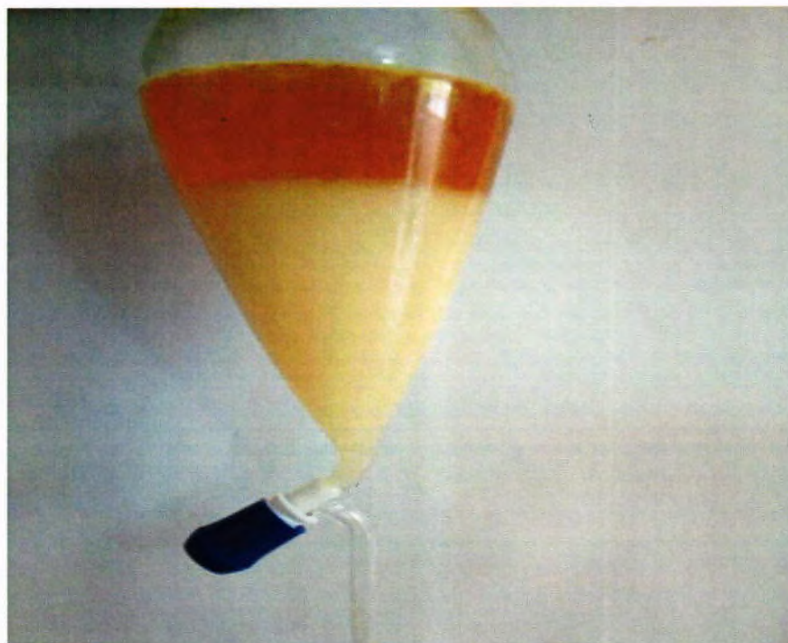
Figure 4.5: Azadirachta indica biodiesel separation
