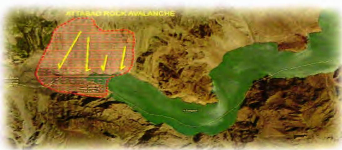
Fig. 3.4. Aerial view of Attabad Landslide Dam along the Hunza River in northern Pakistan. The lake surface partially freezes during the winter (www.googleimage.com)
