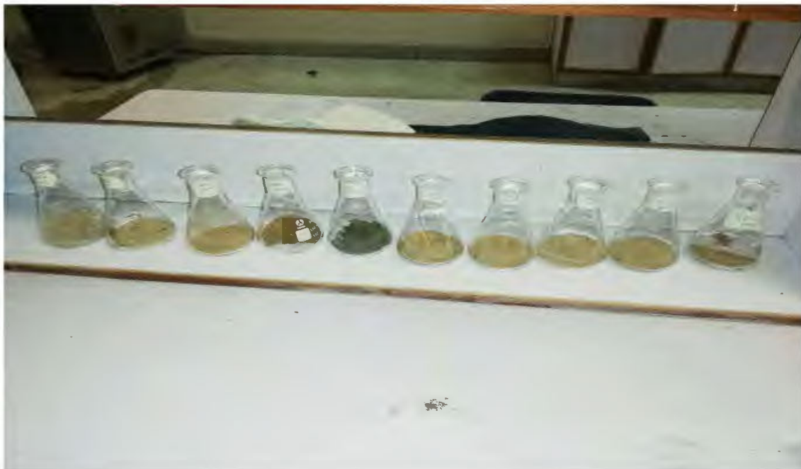
Samples under processing for density separation of Microplastics
