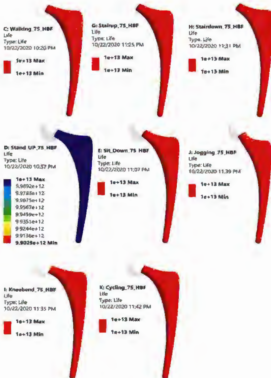
Figure_Apx. A- 9: Fatigue life contour of different activities for body weight of 75 Kg SBF Treated Ti-27Nb.
