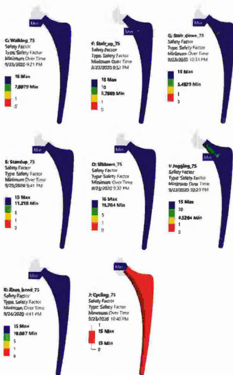
Figure 5-10: FOS contours based on maximum equivalent stress theory for all activities (75kg)
