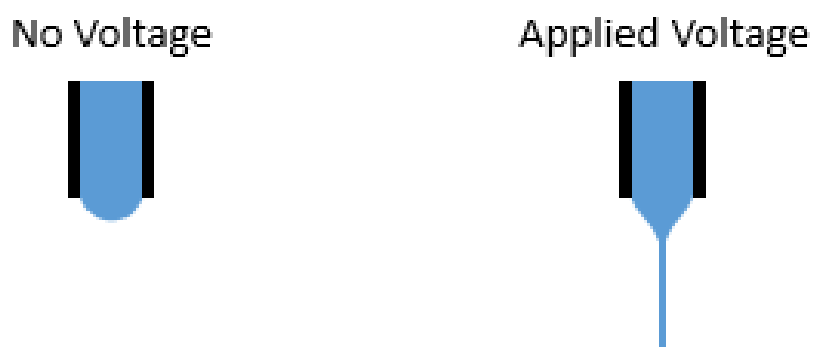
Figure 4.4: Taylor cone formation with and without a potential difference [153].
