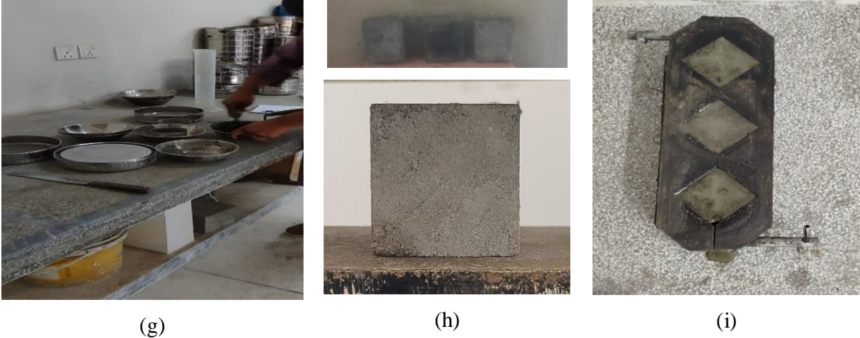
Figure 3.2: Raw Material Testing (a),(b) Cement (c) Sand Specific Gravity (d),(e),(f) Cement Consistence (g)(h)(i)Compressive Strength Cuve
