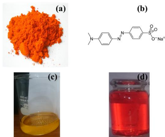
Figure 1.9 (a) Methyl orange in powder form, (b) chemical structure of methyl orange, (c) aqueous solution of methyl orange, and (d) aqueous solution of methyl orange at pH 4 (acidic).
