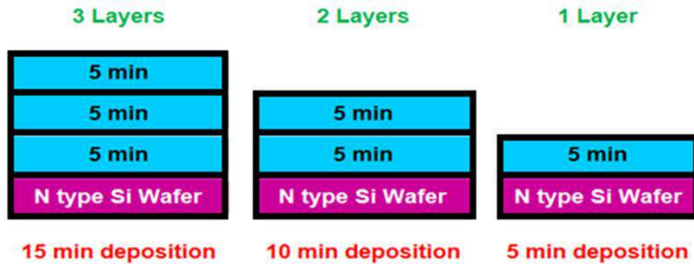
Figure 2.9: Representation of 1, 2 and 3 layer films deposited at X=6 cm.
