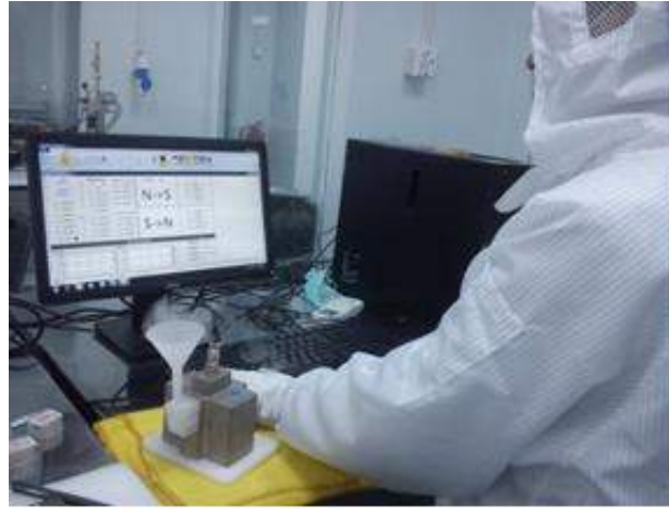
Figure 2.16: Hall effect measurement setup.
