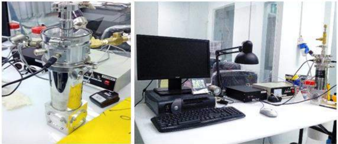
Figure 2.15: IV Measurements under vacuum.
