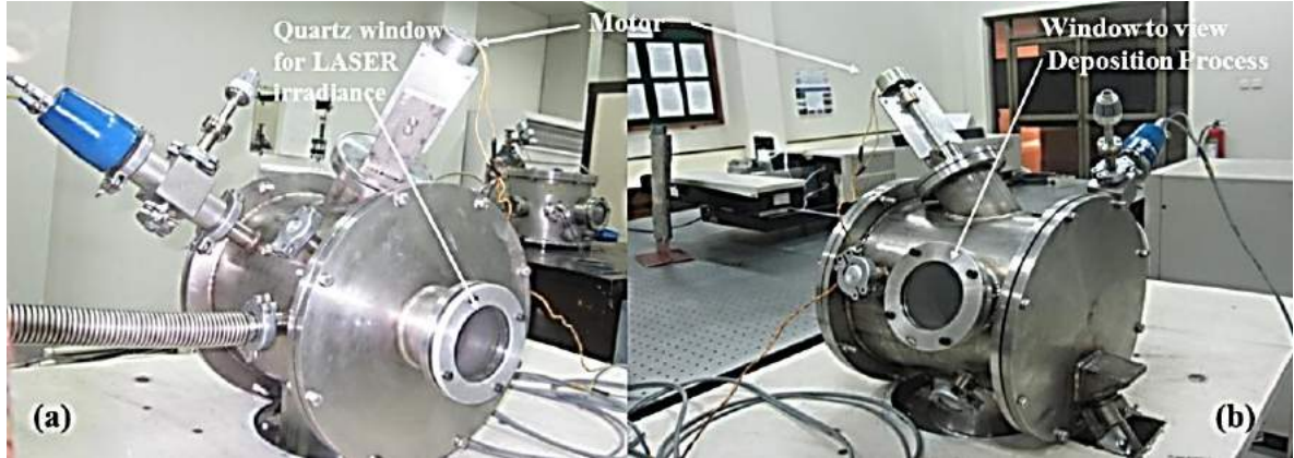
Figure 2.5: Photograph displaying front (a) and rear view (b) of Deposition Chamber.
