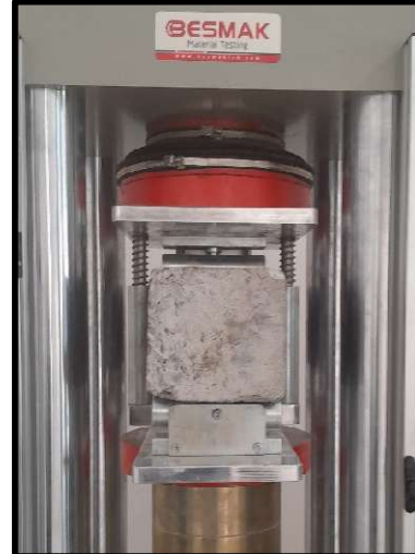
Compression test of Concrete Cube
