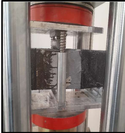
Flexure Test of beam
