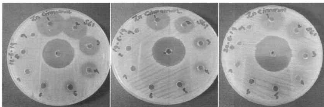
Figure No. 3.62: Photographs of Zone of inhibition of ZnNPs synthesized in the presence of C. zeylanicum bark extract against S. aureus ATCC: 6538 (Gram positive bacterial strain)
