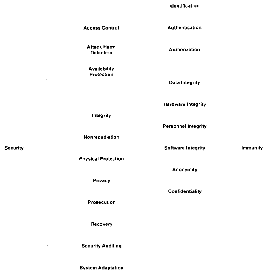
Figure 2.1: Decomposition of Software Security into Security Attributes and Sub-attributes [6]
